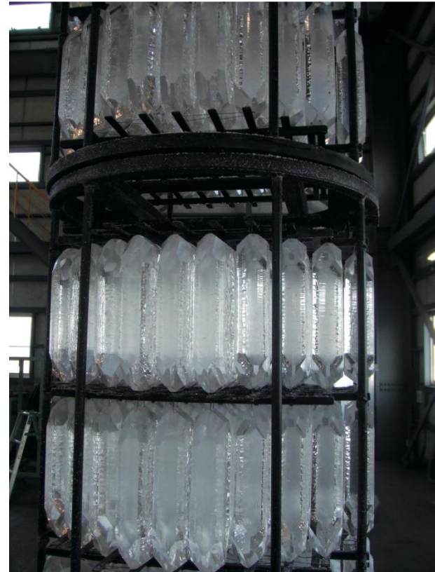
Grown quartz bars in an autoclave
